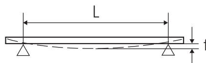
Picture 1: Calculation of loads, f = maximal deflection, L = length
