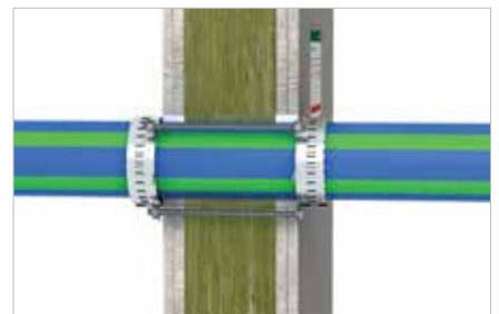
■ Aquatherm Green pipe penetration through a flexible wall construction \geq 100 mm
