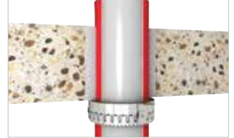
■ Built-in situation ceilings \geq 150 mm
