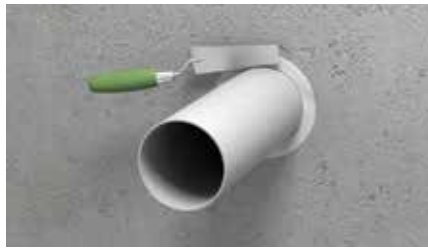
2. Close the gap with loose mineral wool and seal it with a gap filler like Walraven Pacifyre® A acrylic sealant, Pacifyre® H hybrid sealant or Walraven Pacifyre® FPM fire protection mortar (fill depth = 10 mm).
