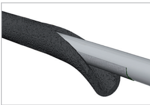
Insulate over both plastic pipe and pipe reinforcement
