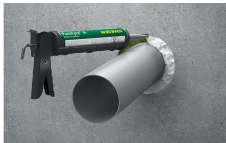
2. Close the gap with loose mineral wool and seal it with Walraven Pacifyre® A Acrylic Sealant (fill depth = 10 mm).
