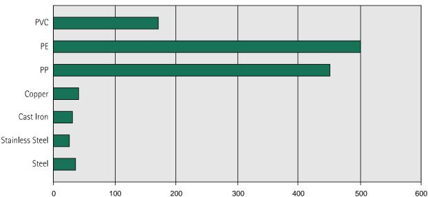
Pipe length: 50 meter, Temperature difference: +50 °C
