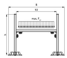
Walraven Strut T-shape Base Plate Walraven RapidStrut® Channel (BUP1000) Walraven Strut Connector 90° (BUP1000)
