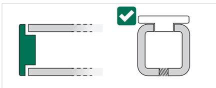
Fit the rail or cantilever arm with a BIS Rail End Cap (656 6 0XX) for clean finishing of rail end and to cover all burrs.
