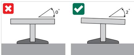
To make sure water runs off freely, place the BIS UltraProtect® 1000 parts at an angle of at least 2°.
